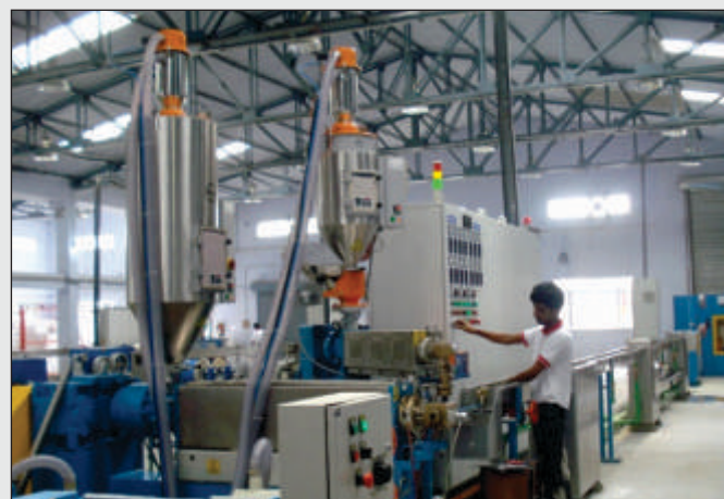
65 / 40mm High Speed PVC Extruder
