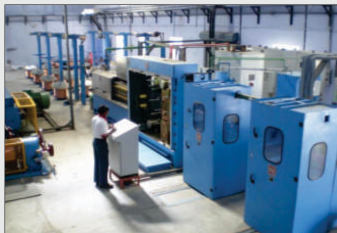
16 Wire High Speed Wire Drawing Machine NEIHOFF - Germany
